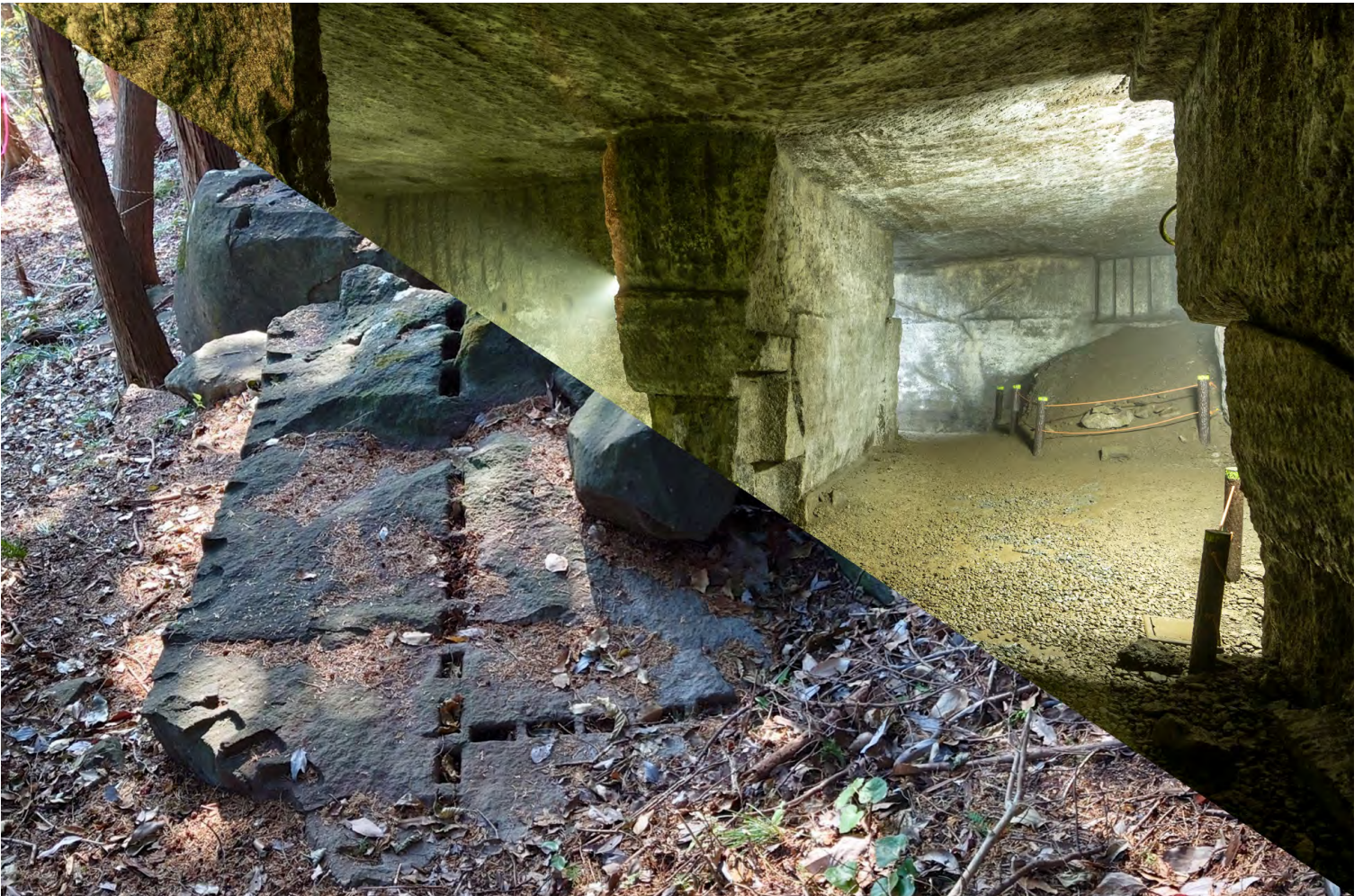
Composite image of quarry remains in the South Fuji–Izu Peninsula area: surface quarry blocks with wedge marks and an underground stone quarry (photo provided by author; image used under commercial-use rights licensed to the association)
