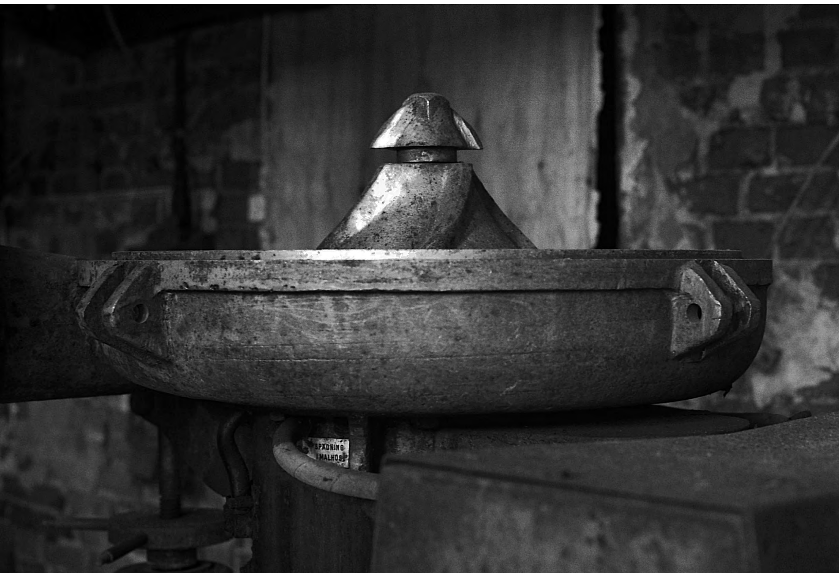
A detail of Krima Moulator. It's a refiner for grinding wood chips, manufactured by a Swedish company now called Cellwood Machinery. Tolkkinen, Porvoo, Finland, August 2013.
