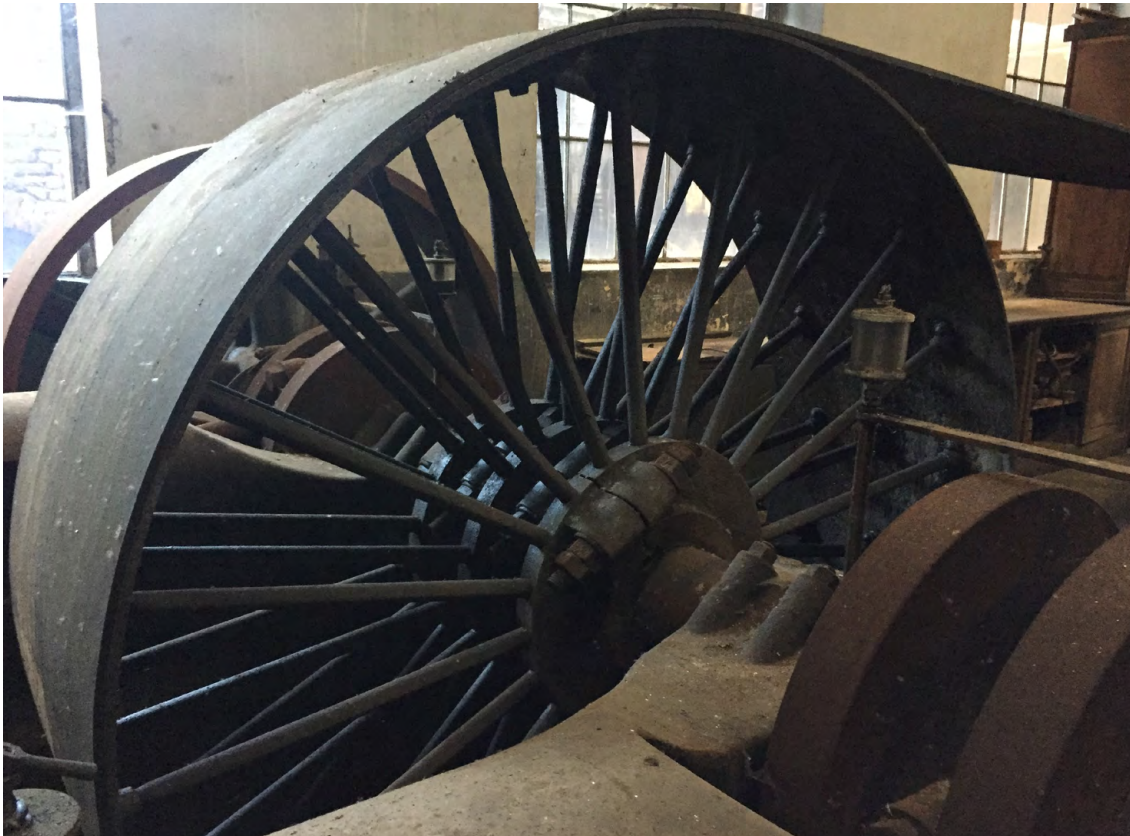
Detail of a steam engine in the power hall of Le Solvent Belge in Verviers, used until recently for the washing and processing of wool by the Traitex company (photo by Patrick Viaene, 2017)
