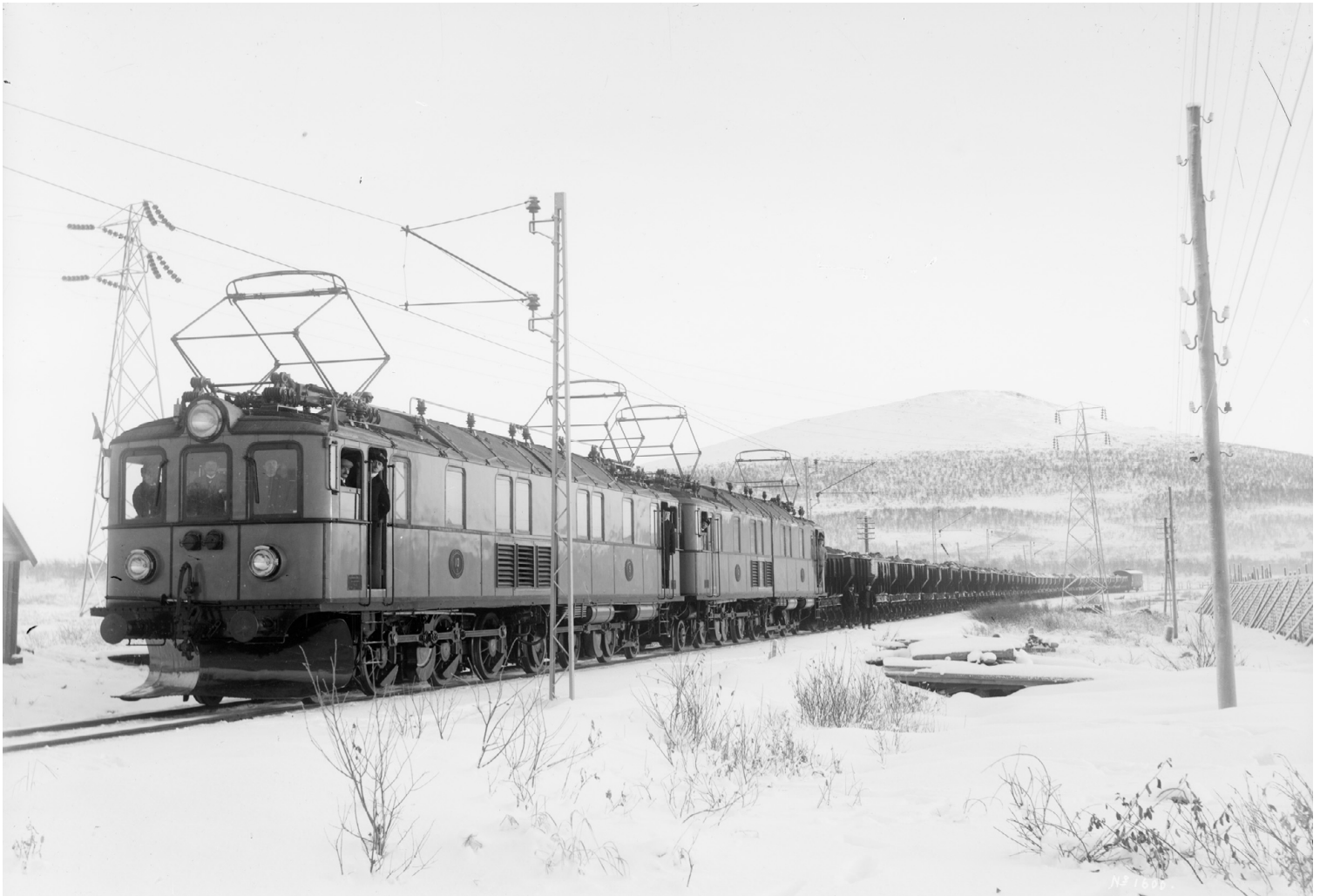
Two Oa-series double-locomotives hauling 30 iron-ore wagons during the test-period in early 1915. The type Oa locomotives were built by Siemens but were assembled in Sweden (photo by Borg Mesch, Kiruna kommun)
