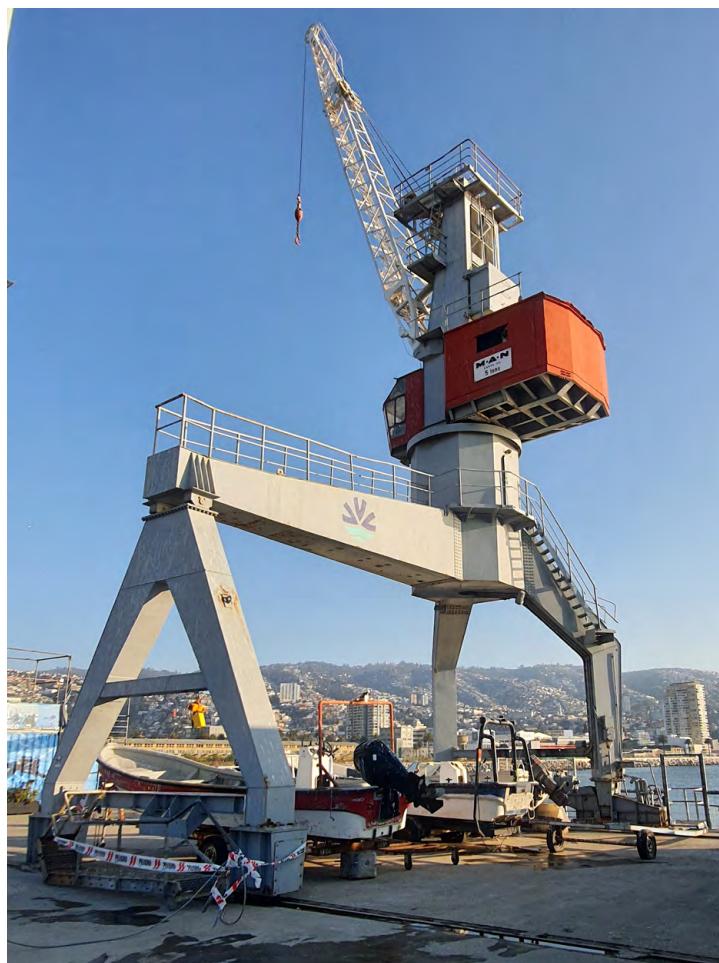
Valparaíso, Muelle Barón. Harbour crane from Germany by MAN, built in the second half of the 1960s and now preserved with the original lifting hook – repair in the scientific sense of industrial heritage conservation (photo by author)
