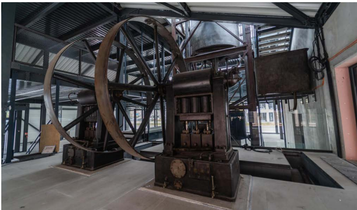
Hydraulic power station with one of the few remaining raised weight accumulators in mainland Europe. Photo: Julia Markiewicz
