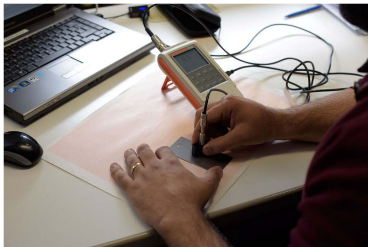
Measuring of the thickness of coatings in the laboratories of German Mining-Museum Bochum. Photo: Helene Grebe
