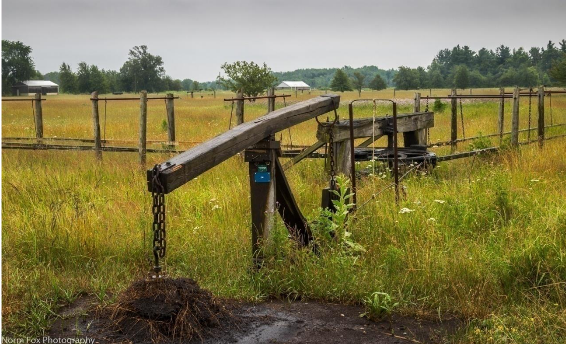
A part of the jerker line system which conveys pumping motion from the central power to the wells. (© Fairbank Oil)
