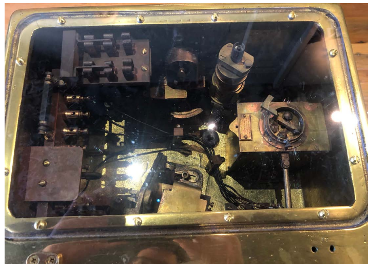
The Type 421 Echometer in Georgetown [South Carolina Maritime] Museum. Its construction of primarily brass and copper helped to preserve it. Perhaps the greatest curiosity: a tag that explicitly forbids bringing the instrument into France.
