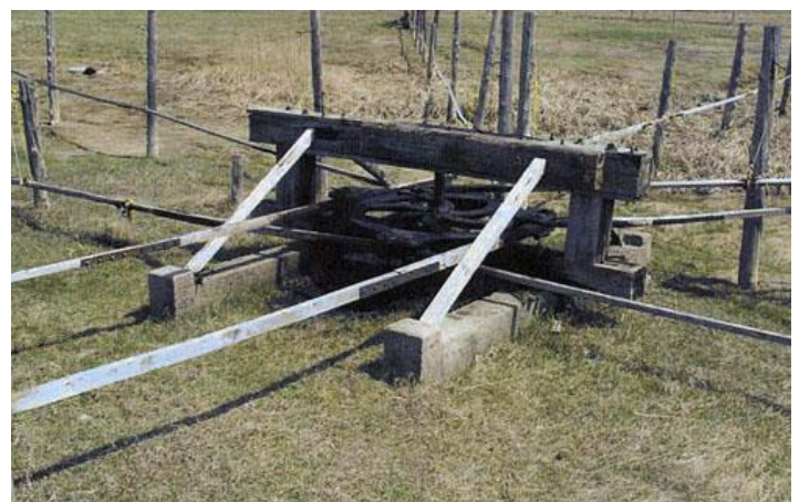
The conserved jerker-line system at Oil Springs, Ontario, was devised so a single steam engine could operate multiple pump jacks pumping oil, with a contemporary derrick in the background. First Commercial Oil Field National Historic Site of Canada. Photo: Parks Canada Agency, A. Roos, 2005.
