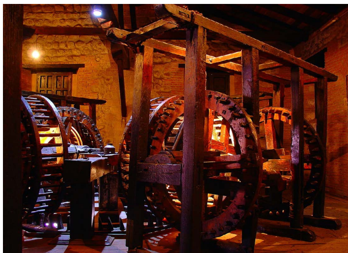
Silver stamping machinery in the Casa Nacional de Modeda in Potosí, Bolivia. Photo: Martin St-Amant - Wikipedia - CC-BY-SA-3.0
