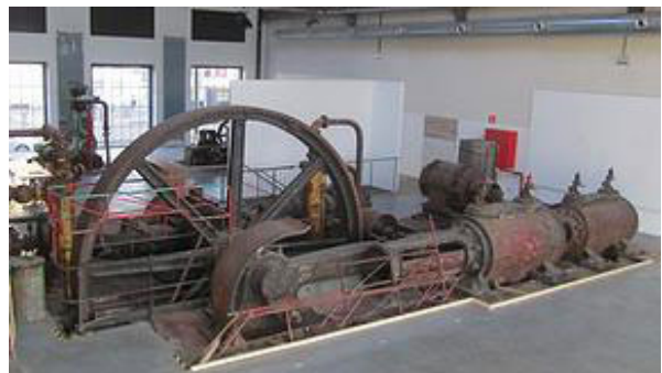
The plant includes a horizontal Carels et Frères steam machine. The site is open for visits by appointment in French, English, Dutch and German.
