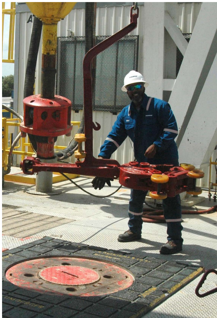
Schlumberger employee and tour guide Deon at the 1988 Genesis Test Drilling Facility explains the power tongs. The tour provided a view of present-day technology. It is a 142-ft.-tall, cantilever-type, skiddable, land-drilling rig used as a training tool and product testing platform for various tests including mud viscosity and flow, and downhole tool vibration and rotation. Photo: John Reap
