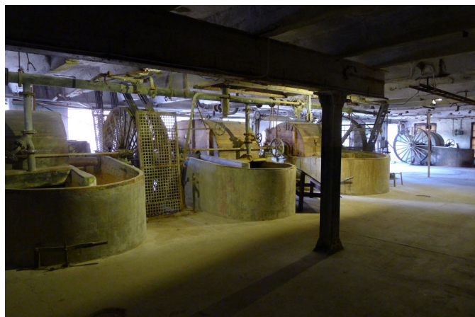
Hollander beaters with their drive chain inside the mill.
