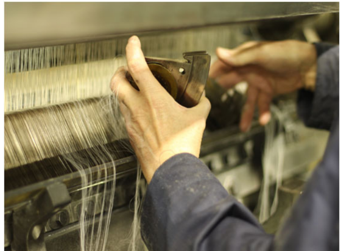
Installing carriages in the machine, Cluny Lace, 2013
