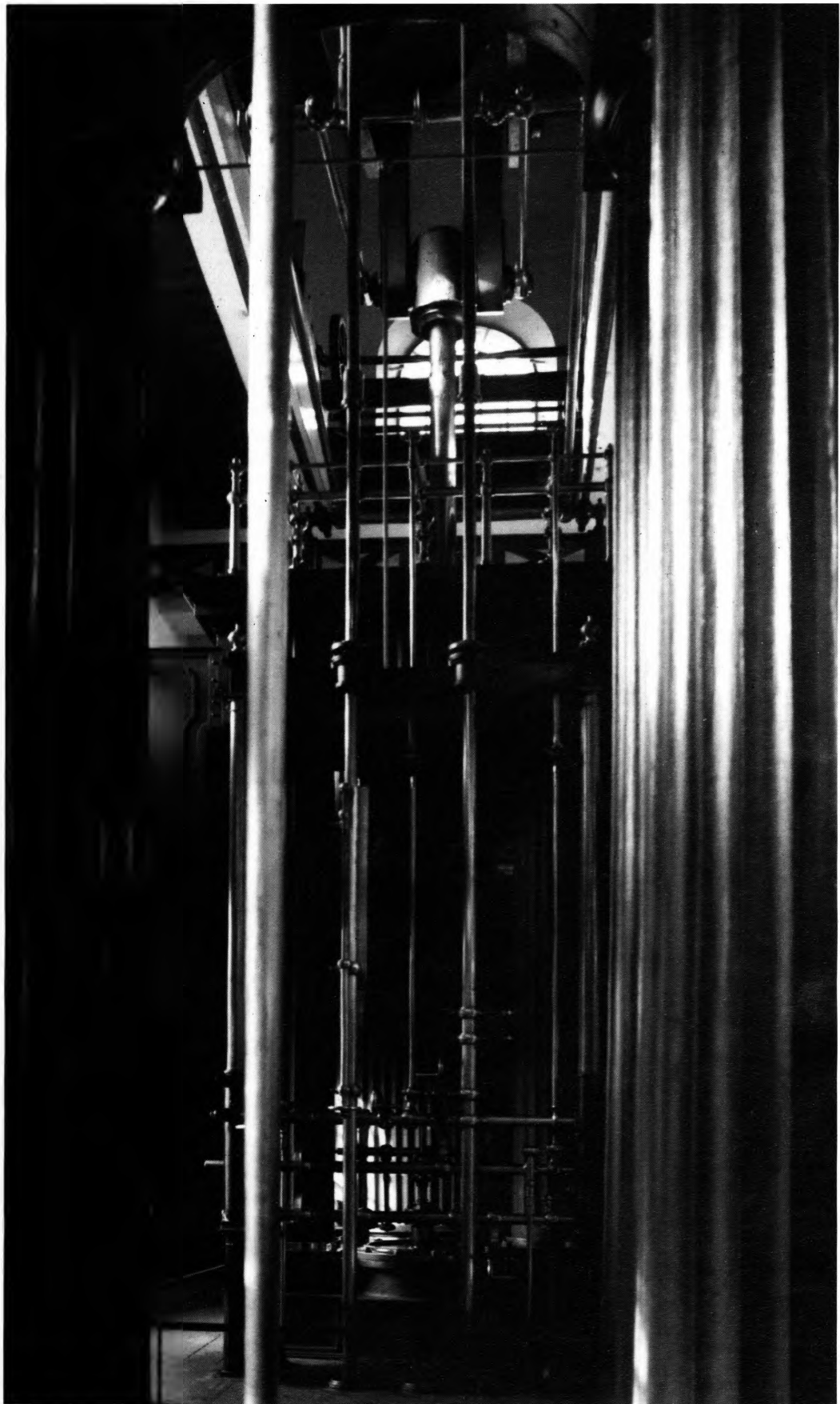
TICCIH2000 delegates visited the Kew Bridge Steam Museum and saw this 90-inch cylinder Cornish beam pumping engine in operation. This engine was manufactured by Sandys, Carne and Vivian of Hayle, Cornwall for the Grand Junction Water Works Company at Kew in 1846. It is one of several engines under the care of the Kew Bridge Engines Trust at their Museum of Water in west London. Photograph by Dick Fillery, supplied by John Porter, © Kew Bridge Engines Trust.
