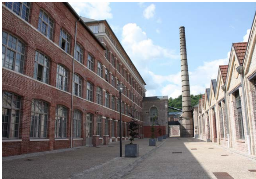
Gasse & Canthelou factory. Situated in the centre of the city, this factory specialised in weaving and finishing of woollen cloth. A 1842 timber-framed building with an 1882 metal framed addition and a new north-lit weaving shed added in 1918. The factory has been converted into housing and was awarded the Auguste Perret Prize in 2010.
