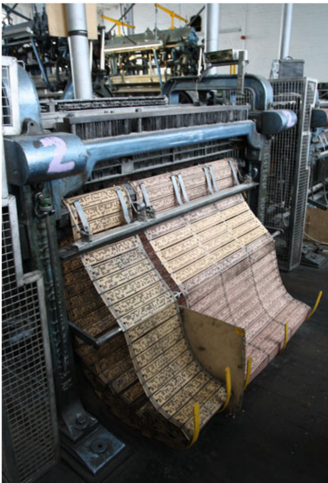
Jacquard cards that control the movement of the threads in the Leavers Machine, Cluny Lace, 2013.
