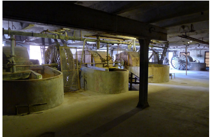
Hollander beaters with their drive chain inside the mill.
