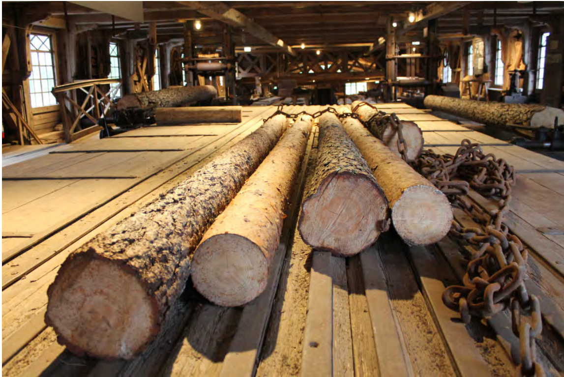
Log bed, log carriages (1880, Bolinder) and frame saws (1882) at the Makkarakoski sawmill museum. The sawmill was built in 1875. © Hanna Jaakola 2014
