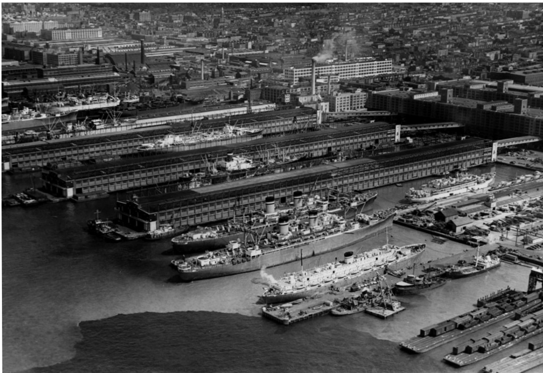
Aerial view of the Brooklyn Army Terminal during World War II - its busiest period of operation. Sky bridges and rail lines connected the two 980ft long terminal buildings to enormous sheds straddling each of the four piers, enabling the rapid transfer of goods, equipment and troops between land and sea.
