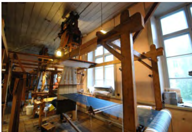
The weaver Sonja Enbuske at work in one of the 170-year old looms. Note the jacquard head at the top
