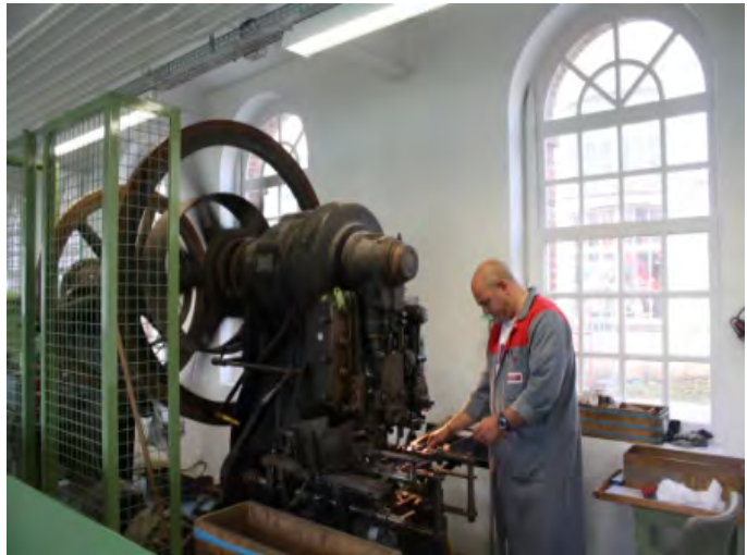
The large press for longer needles. Visitors stand beside skilled industrial needle smiths witnessing the work in progress.
