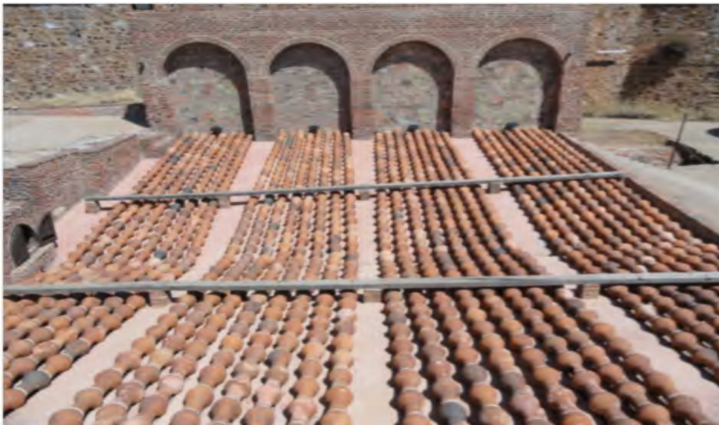
One of the 17th century furnaces for distilling mercury vapour, which was drawn through the lines of clay pots.
