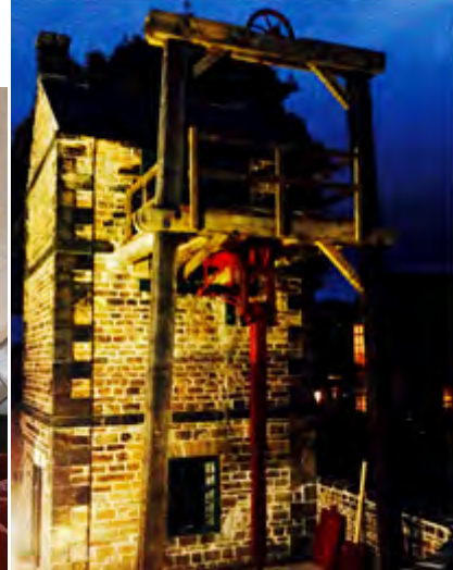
Elsecar pumping engine near Barnsley, the piston ready to go back into the cylinder. © Industrial Heritage Consulting Ltd
