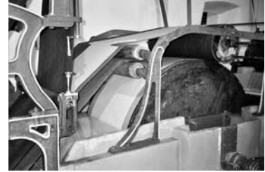
Continuous paper machine of the Picard type in the Munné mill.
