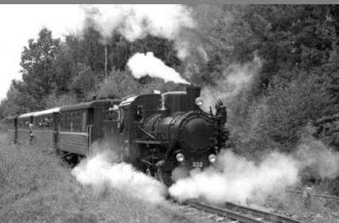
Kc4-332 in full steam running along the last operational narrow gauge (750 mm) railway in the Baltic countries.
