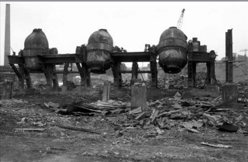
Blasted out. Three cold Bessemer converters from Rolf Hohemann's international study of the conservation of iron and steel works.
